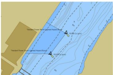
AS OF OCTOBER 2019, VERDANT POWER, UNDER THE ABOVE FERC PROJECT LICENSE AND IN COORDINATION WITH THE US COAST GUARD AND NOAA, HAS ESTABLISHED TWO PRIVATE AID TO NAVIGATION (PATON) BUOYS AT THE RITE PROJECT SITE IN THE EAST CHANNEL OF THE EAST RIVER. THESE BUOYS PROTECT AN ESTABLISHED NAVIGATION EXCLUSION ZONE {AS SHOWN IN ENC US5NY1DE} THAT DIRECTS ALL WATER-BASED TRAFFIC TO USE THE ESTABLISHED VESSEL TRANSIT AREA TO THE EAST OF THE BUOYS.
